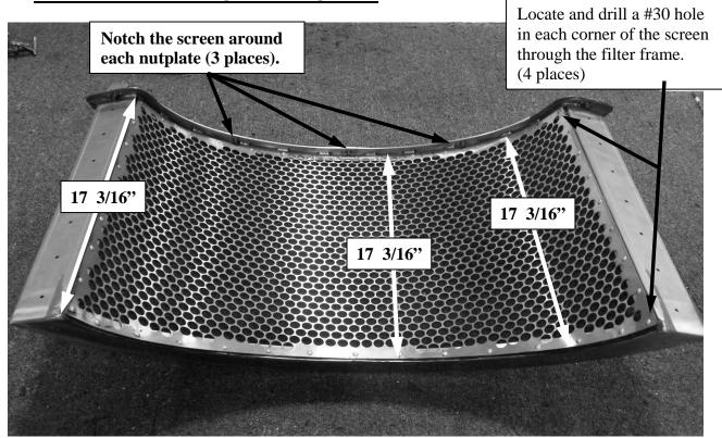
□ On the wide curved band on the forward side of the frame, drill the two #30 holes that are shown in the picture below. Use a flexible tape measure oriented perpendicular to the side channels of the frame. Start the measurements from the face of the side channel as shown below. Repeat this for both the left and right sides, resulting in a total of four #30 holes.
