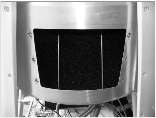
This picture shows the view through the access opening in the bottom of the lower plenum cover. This picture is with the access cover removed, exposing the filter element for cleaning or close-up inspection.
