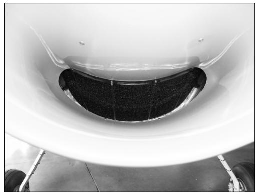
This picture shows the view down the engine inlet looking toward the Brackett foam air filter. From this view, the pilot/mechanic can inspect the filter during preflight for proper installation, excess dirt/debris, or any damage to the filter or filter frame.
