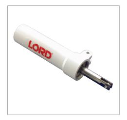
The Parker LORD® fluid-free shimmy damper offers high-performance damping and vibration control with a zero-maintenance design. Instead of using fluids to resist motion, the shimmy damper features a unique elastomer formulation to absorb nose wheel shimmy. Since there is no fluid, this damper will never leak.
