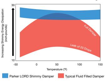
Parker LORD surface effect dampers operate consistently in the -40° to 150° Fahrenheit range while traditional hydraulic dampers only provide peak energy dissipation in the 20° to 80° Fahrenheit temperature range.
